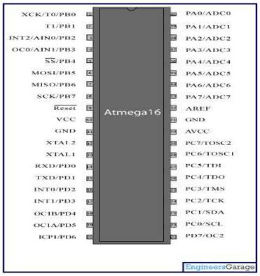
ATmega16 is an 8-bit high performance microcontroller of Atmel's Mega AVR family with low power consumption. Atmega16 is based on enhanced RISC (Reduced Instruction Set Computing, Know more about
